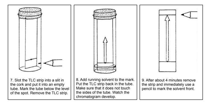
10. Measure the distance run by the solvent front and by each of the pigments. All measurements should be made from the centre of the original spot to the front of each pigment spot.
